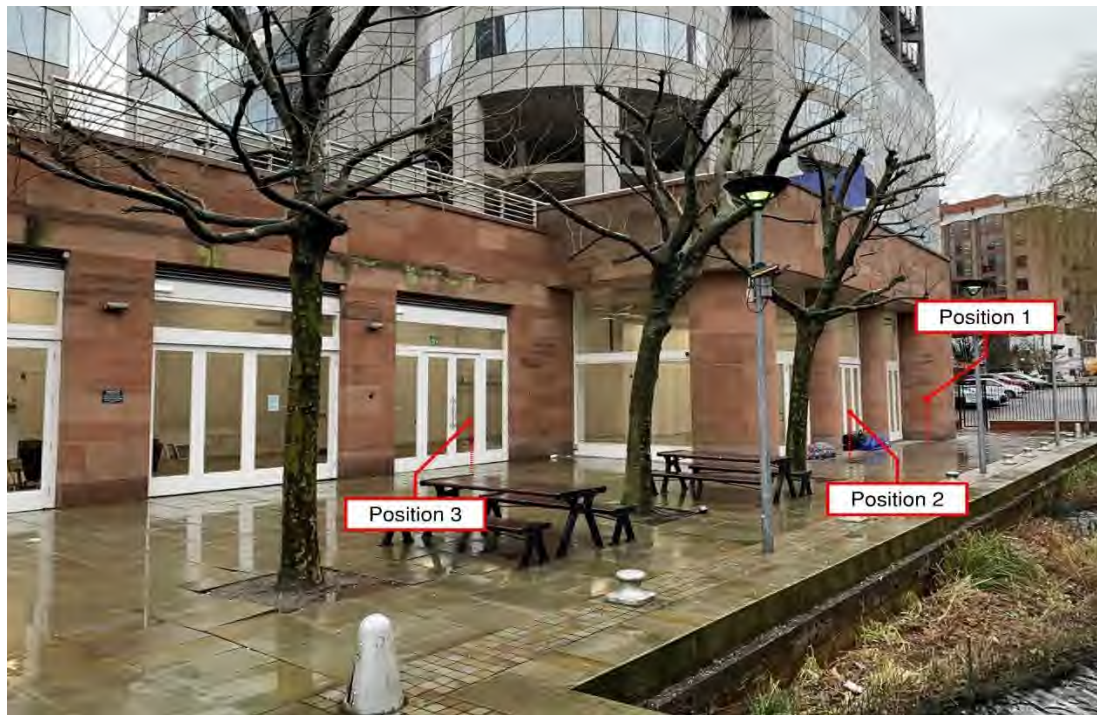
Figure 3 – Noise break-out measurement positions
